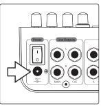
3. Connect the included power supply to the appropriate wall socket and then to the Monitor Station V2's rear-panel power input.
