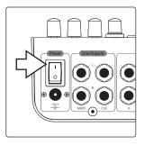
4. Turn on the Monitor Station V2's power by pressing the "|" symbol at the top of the Power switch.
