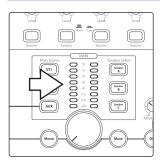
By default, the Monitor Station V2's LED meters are calibrated so that the red 0 VU LED illuminates when the selected source signals reach +10 dBu. This can be changed so that 0 VU references +4, +10, or +18 dBu.
