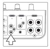
**Analog audio device with RCA outputs.** Connect the device's outputs to the Monitor Station V2's rear-panel unbalanced RCA AUX L/R IN jacks.
