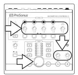
1. Zero the Main Output level, Talkback level, Cue output, individual headphone level, and Dim attenuation knobs by turning them fully counterclockwise.
