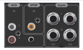
**ST1 L/R:** Connect the left and right channels of your primary stereo source to these balanced ½"TRS jacks.
