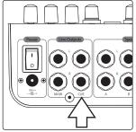
2. Connect the inputs of the headphone amplifier to the Monitor Station V2's Cue L/R Line Outputs.
