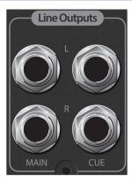
**Main L/R Line Outputs:** Monitor Station V2 passes input audio sources directly to the Main L/R Line Outputs. These outputs derive their signal directly from the currently selected Main input sources and are unaffected by the Main level-control knob and the Mono, Mute, and Dim buttons. Connect these balanced ¼"TRS jacks to the inputs of a stereo device.
