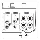
2. Connect your primary audio source (computer audio interface, mixer, or other stereo source) to the balanced ¼"TRS ST1 L/R inputs on the back of your Monitor Station V2.
