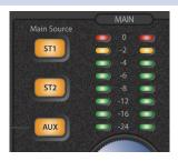
**Main Source Buttons:** The Main Source buttons select the audio for the Speaker Output jacks, the Main L/R Line Outputs, and any headphone amplifiers whose Source switch is set to its Main position (up).
