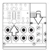
1. Zero the Monitor Station V2's front-panel Main Output Level knob and rear-panel Speaker A Out trim by turning them fully counterclockwise.
