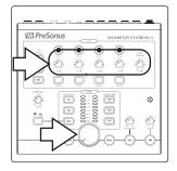
Zero the Monitor Station V2's front-panel Main Output Level knob, the Cue Output knob, and the individual headphone Level knobs by turning them fully counterclockwise.
