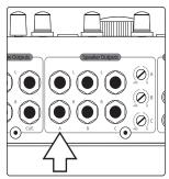
2. Connect your primary monitoring system (such as a pair of powered nearfield reference monitors) to the Monitor Station V2's A L/R Speaker outputs.
