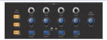
The Cue section of the front panel allows you to manage the Monitor Station V2's Cue system and control its four individually controllable headphone outputs. Each output has its own input selector and its own volume control.
