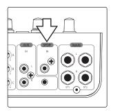
**Digital audio device with S/PDIF output.** Connect the source device's S/PDIF output to the Monitor Station V2's rear-panel RCA (coaxial) S/PDIF input. The Monitor Station V2 supports sample rates of 44.1, 48, 88.2, and 96 kHz.
