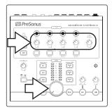
1. Zero the Monitor Station V2's front-panel Main Output Level knob, the Cue Output knob, and the individual headphone Level knobs by turning them fully counterclockwise.
