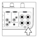
3. If you have a secondary stereo audio source or cue audio source—such as other interface outputs or the auxiliary outputs of your mixer—connect it to the balanced ¼"TRS ST2 L/R inputs.
