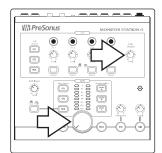
Zero the Main Level and Cue Output knobs by turning them fully counterclockwise.
