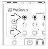
Connect headphones to any one of the Phones outputs and select Cue as the source by pressing the corresponding Source button so that it latches in its down position.
