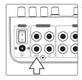
2. Connect the inputs of the external device to the Monitor Station V2's Main L/R Line Outputs.
