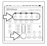
1. Zero the Monitor Station V2's front-panel Main Output Level knob, the Cue Output knob, and the individual headphone Level knobs by turning them fully counterclockwise.
